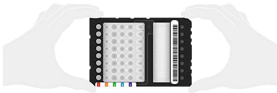
Figure 3. Proper handling and placement orientation of an Ionic fluidic chip.
